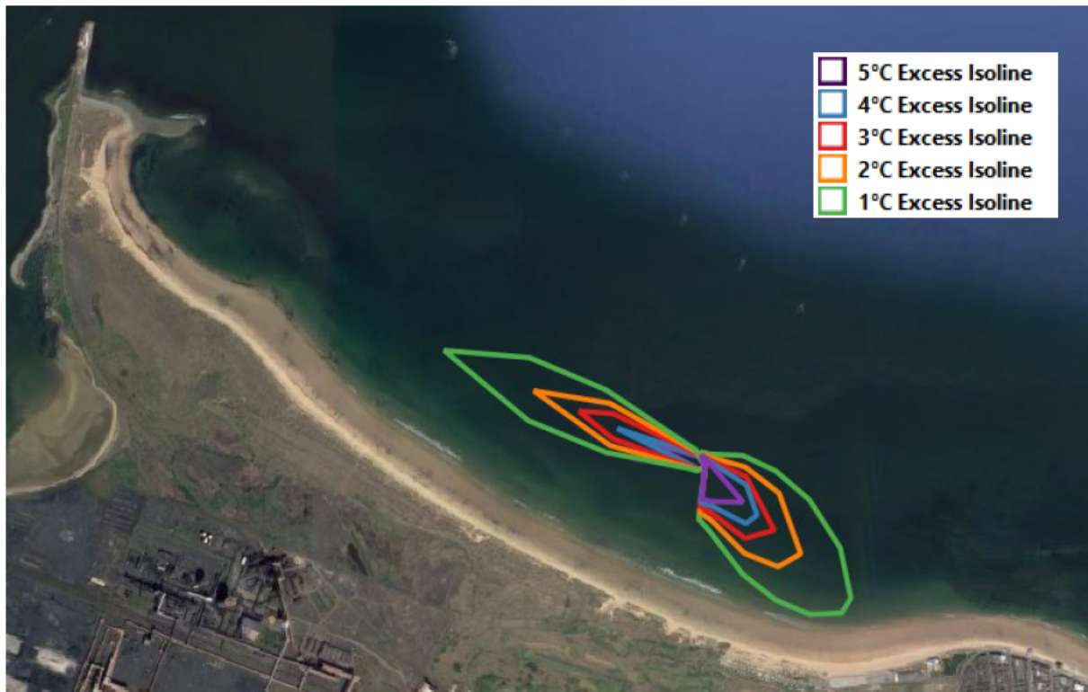
Figure 16. Excess temperature isolines during a neap tide under normal discharge conditions.
